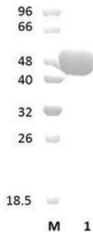
Figure 1. SDS-PAGE analysis of GFP-CBM30 was conducted in (Lane 1), employing a 14% polyacrylamide gel. The enzyme exhibits a band corresponding to a molecular weight of approximately 50,67 kDa. Lane M contains a Protein Marker for reference.
