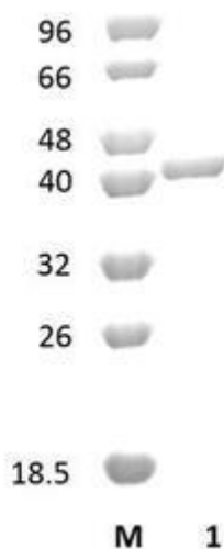
Figure 1. SDS-PAGE analysis of ZgAga16D (GH16) was conducted in (Lane 1), employing a 14% polyacrylamide gel. The enzyme exhibits a band corresponding to a molecular weight of approximately 42,49 kDa. Lane M contains a Protein Marker for reference.
