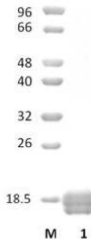
Figure 1. SDS-PAGE analysis of CBM4 was conducted in (Lane 1), employing a 14% polyacrylamide gel. The enzyme exhibits a band corresponding to a molecular weight of approximately 17,80 kDa. Lane M contains a Protein Marker for reference.
