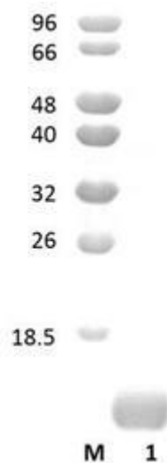
Figure 1. SDS-PAGE analysis of CBM2 was conducted in (Lane 1), employing a 14% polyacrylamide gel. The enzyme exhibits a band corresponding to a molecular weight of approximately 12,65 kDa. Lane M contains a Protein Marker for reference.
