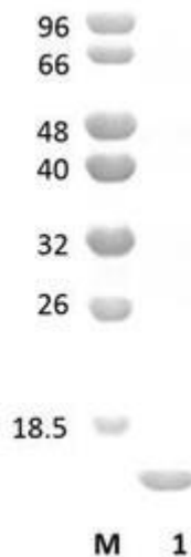
Figure 1. SDS-PAGE analysis of CBM2 was conducted in (Lane 1), employing a 14% polyacrylamide gel. The enzyme exhibits a band corresponding to a molecular weight of approximately 12,90 kDa. Lane M contains a Protein Marker for reference.
