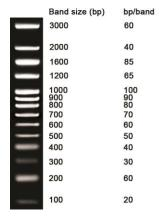
**Figure 1.** Precisely 5  $\mu$ L of NZYDNA Ladder VII were electrophoresed in a 1.5% (w/v) electrophoresis grade agarose (MB027) gel. The gel was buffered with TAE (v/v) and stained with GreenSafe Premium (MB13201).
