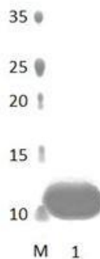
Figure 1. SDS-PAGE analysis of DLG2_3 PDZ Domain was conducted in (Lane 1), employing a 14% polyacrylamide gel. The enzyme exhibits a band corresponding to a molecular weight of approximately 12.98 kDa. Lane M contains a Protein Marker for reference.
